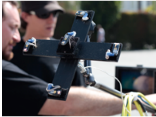
Figure 24: A rigid body designed for use with a PhaseSpace system. Source: Michael Weaver
