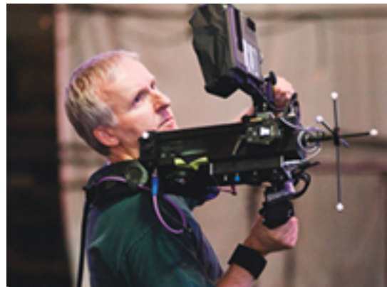
Figure 23: The virtual camera used on Avatar utilized a passive optical tracking system marker configuration. Source: Frank Rose
