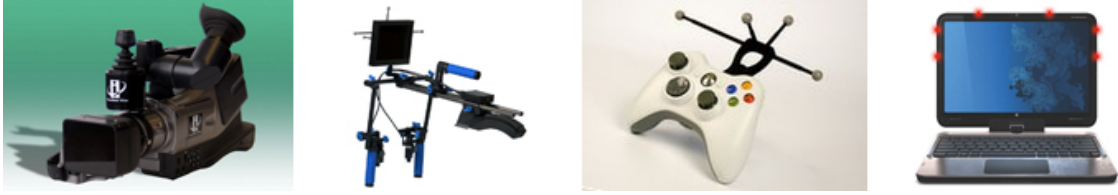
A variety of consumer virtual cameras, from left: Figure 1: Intersense VCam™. Figure 2: NaturalPoint VCS: Pro. Figure 3: NaturalPoint VCS:Mini. Figure 4: PhaseSpace customized HP® TouchSmart.
