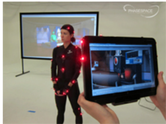
Figure 27: TCam draws from the PhaseSpace virtual camera (above) by embedding markers on the casing. Source: PhaseSpace
