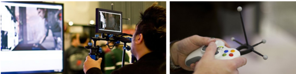
Figures 26: NaturalPoint VCS:Pro (left) provides vital support and camera controls with the use of a shoulder rig, while the VCS:Mini provides a lightweight and more flexible alternative.
