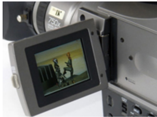
Figure 25: InterSense VCam™ LCD viewfinder with real-time MotionBuilder® feed. Source: InterSense
